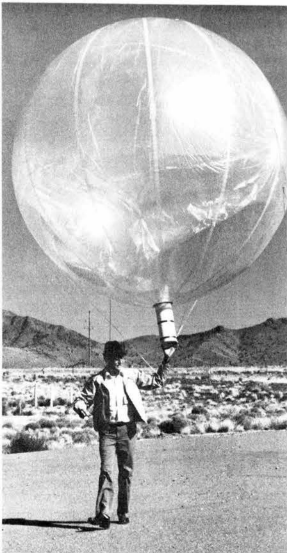
IT GOES UP — AND DOWN — Hugh Church of Applied Atmospheric Research Division 6324 prepares to release a prototype of the Adjustable Buoyancy Balloon Tracer. The division is developing the balloon to help scientists track air flow over a thousand miles or more, gathering data on how atmospheric motion affects acid rain and other forms of long range air pollution.
